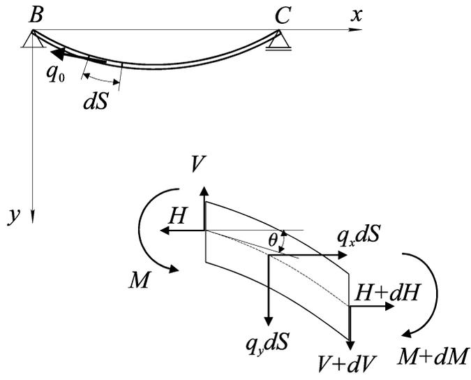
**Figure 1.** Coordinate system and load configuration.
