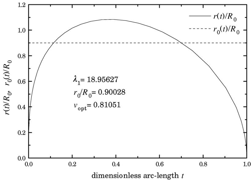
Figure 3. The shape of the optimal column.
